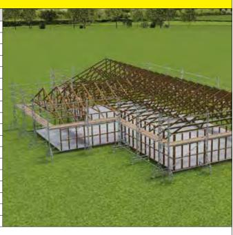
• A comprehensive pack of equipment that includes multiple internal and external corner kits as well as two gated access points.
